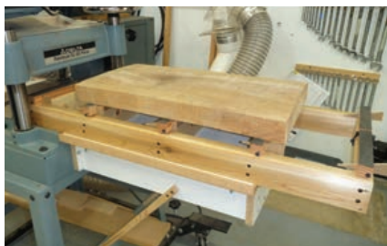
Sledding it – A planer sled does a half-decent job of flattening pieces that are too large for a jointer.
