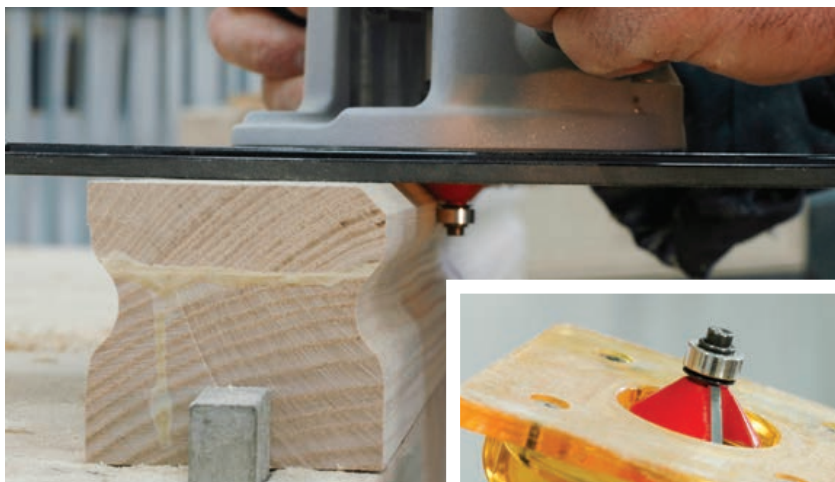
Ease the underside – This step can be done with a chamfer bit or a 1/2" round-over bit for slightly different esthetics.
