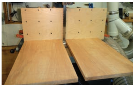
Booking it – The Arbutus pieces are re-sawn on the bandsaw with a high fence.
