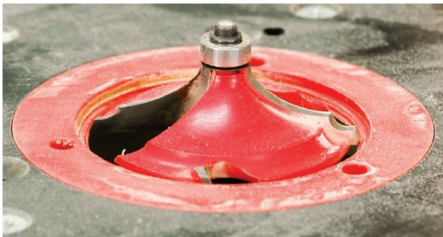
Routing the top profile – This bit will give the rail its decorative appearance.
