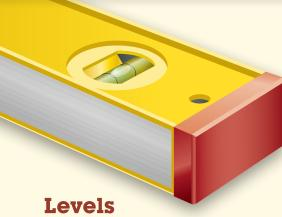
Though not often used for furniture making, a level is critical when doing most home improvement work. Different lengths are available, and having one short level and one longer level on hand is advisable.
