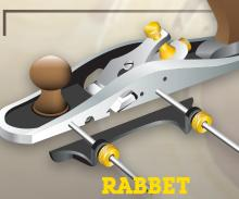
Varying sizes. Used to cut rabbets to a certain depth. They have a depth guide to stop cutting the joint at a certain depth, as well as a fence to cut rabbets at a certain width. They tend to look similar to most bench planes. The blade extends flush with at least one outside edge of a rabbet plane, and they are sometimes available in both left or right hand models.
