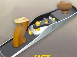
12" - 15" long, Versatile and are great for many tasks around the workshop like removing machine mill marks and prepare the surface for finer hand planes to take over.
