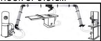
Ideal for connecting two machines to a dust collector
